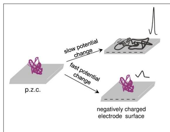
**Scheme 1** Effect of  $I_{\text{str}}$  intensities (current densities) on CPS response of native serum albumin. In CPS the rate of potential changes increases non-linearly with current density. Serum albumin does not show any sign of denaturation close to the potential of zero charge (p.z.c.), however denatured after its exposure to negative potentials.
