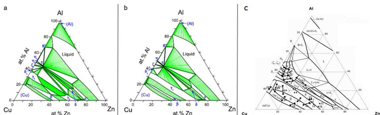
**Figure 1:** Isothermal section of Al-Cu-Zn phase diagram at 550 °C a) theoretical phase diagram with two-phase field [6] b) theoretical phase diagram with the  $\gamma$ \_phase region is continuous from the Al-Cu side to the Cu-Zn side [3] c) published experimental phase diagram [2] with superimposed our experimental results
