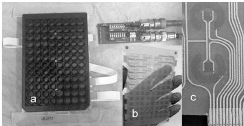
**Figure:** a) Encapsulated OECT 96 well microplate for electrogenic cells cultivation and investigation with power source and signal amplifier b) foil with the all screen printed OECT array c) detail of the OECT with PEDOT:PSS printed channel and gate electrode.
