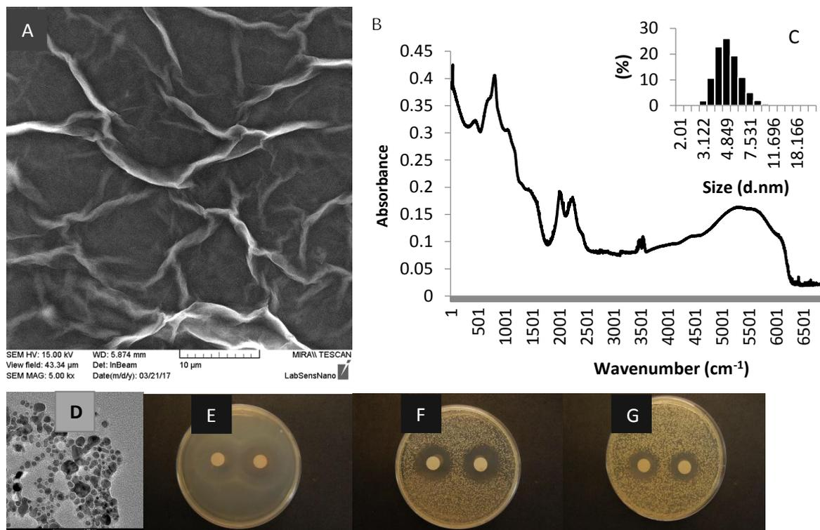
**Figure 1.:** (A) SEM image of GO; (B) ATR-FTIR spectrum of GO; (C) Dynamic light-scattering (DLS) spectrum of silver nanoparticles dispersions—size distribution by number; (D) TEM image of Ag nanoparticles; (E), (F), (G) photos of inhibition zones of the highest applied concentrations of silver nanoparticles on *S. aureus*, *E. coli* and MRSA.
