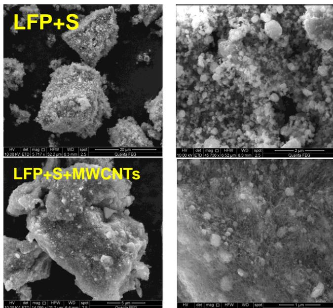
**Fig. 1** SEM images showing the morphology of the S-LiFePO<sub>4</sub> sample (up) and S-LiFePO<sub>4</sub>-MWCNTs sample (down).
