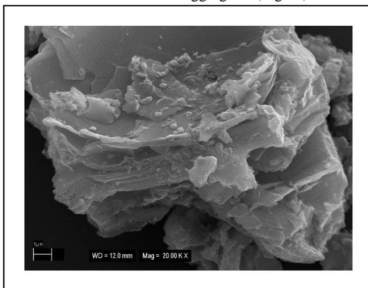
**Figure:** Representative SEM image of Ti<sub>3</sub>C<sub>2</sub>T<sub>x</sub> sonicated for 1 min. Magnification: 20,000×.
