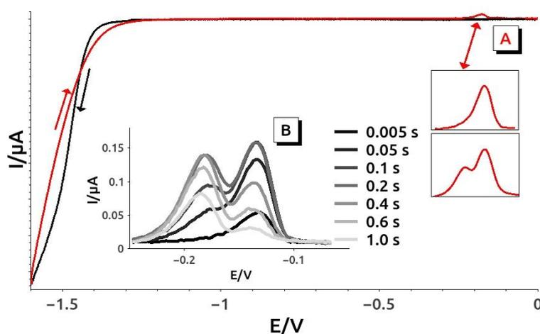
**Figure:** A) Cyclic voltammogram at SMDE with image of two possible shapes of guanine oxidation signals; B) the effect of time of reduction (at -1.45 V) on the shape of GODP; sample d(GGG), concentration 0.72  $\mu\text{M}$ , acetate buffer, pH 4.5, scan rate 0.9 V/s, step 2 mV, in CV vertex potential -1.6 V.
