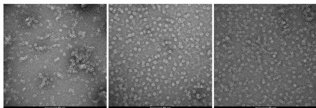
**Fig. 2** TEM micrographs of apoferritin (A), freshly prepared ApoElli (B) and ApoElli stored for 1 month at 4 °C (C).
