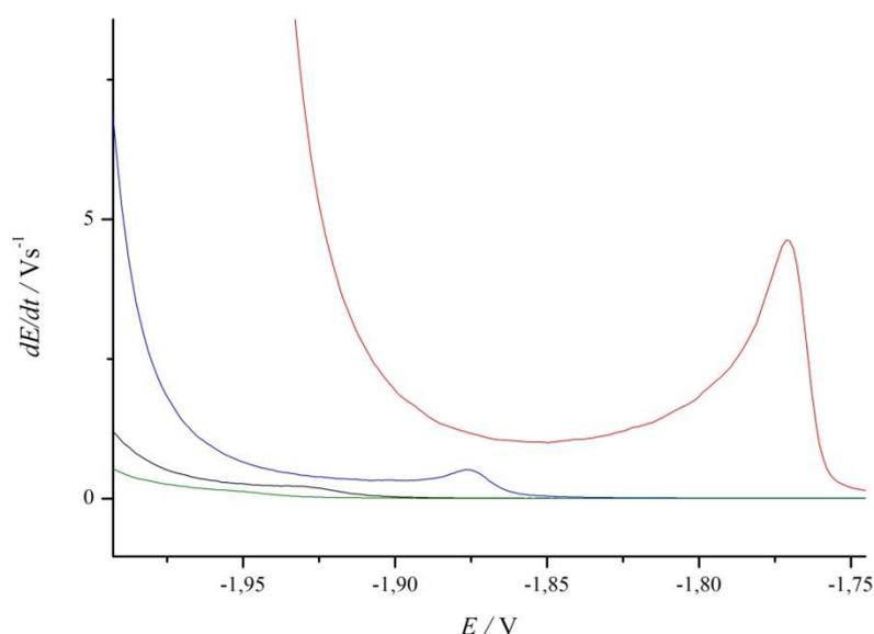
**Figure 1.** CPS voltammogram of four measurements of 60 $\mu$ l EK in solvent PBS with pH=7,24. Deposition potential -1,4V where current was set to -5 $\mu$ A (red), -25 $\mu$ A (blue), -45 $\mu$ A (black), -65 $\mu$ A (green). Duration time was set to 480s.
