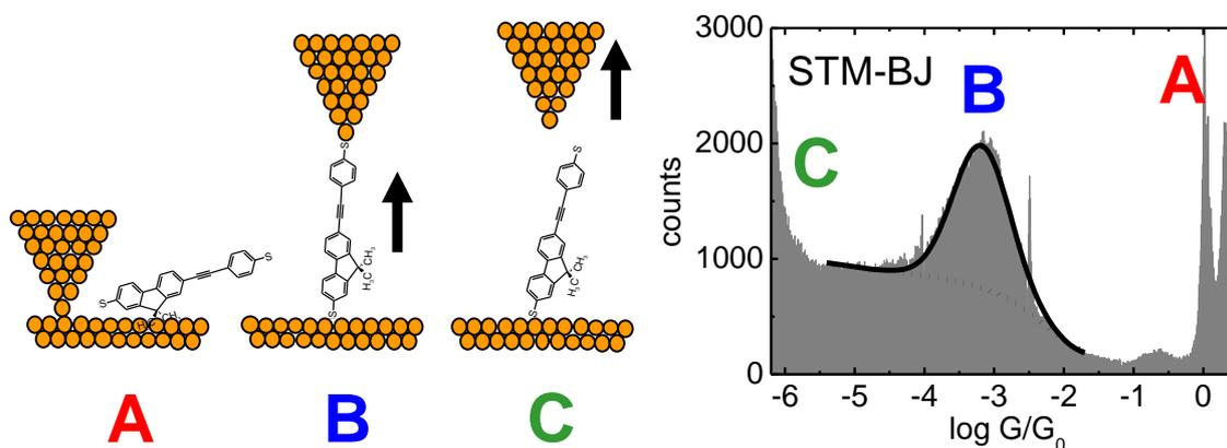
**Figure:** Principle of the Scanning Tunneling Microscopy Break Junction Technique
