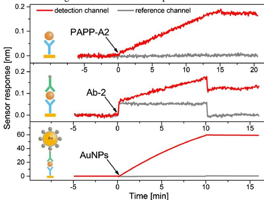
**Figure:** The sensor response corresponding to respective steps of the assay for detection of PAPP-A2 in buffer. Direct detection of PAPP-A2 (top), binding of biotinylated Ab-2 (middle), binding of streptavidin-coated AuNPs (bottom)
