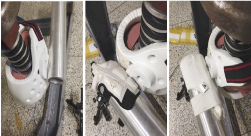
Fig. 3 No footpad condition (left), World Taekwondo Federation-approved footpad (center) and thick footpad (right). It should be noted that the thick pad was commonly employed during taekwondo competitions. However, at the time of its use, no official regulation existed for foot protection
