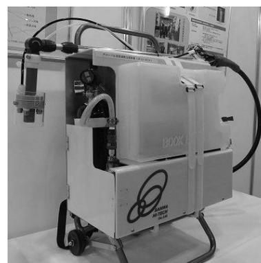
Fig.1 Portable ozone-mist sterilization system
