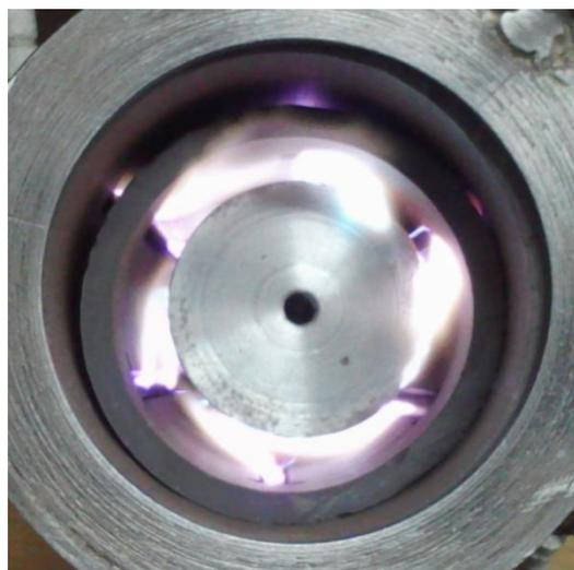
**Fig. 2.** A gliding discharge reactor equipped with six high voltage electrodes.
