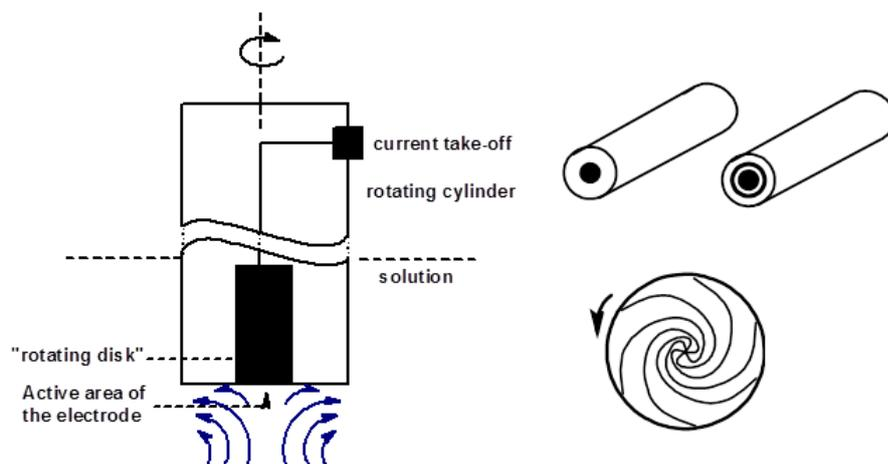
The resulting voltammogram has the shape of the sigmoidal wave, the height of which represents the analytical signal. To understand the processes taking place in the RDE experiment a notion of the layer of solution immediately adjacent the electrode, which moves along with it, is important. Through this layer the transport of the test compound proceeds by diffusion. From the electrode point of view this layer is stationary (stagnant layer).
