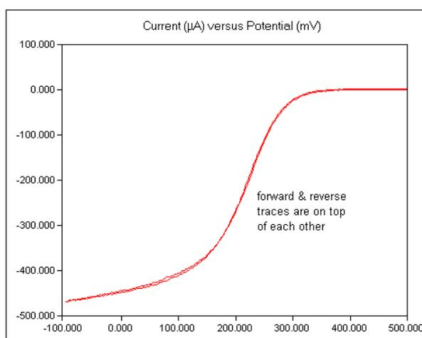
**Figure 1: Model hydrodynamic voltammogram of ferricyanide**
