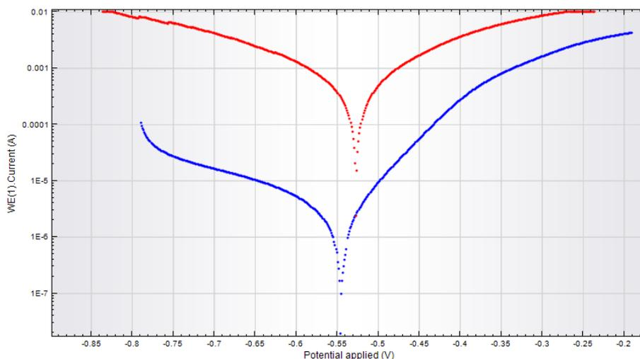
**Fig. 2:** Real voltammograms of mild steel samples in different environments: saline solution (blue), 0.1 M H<sub>2</sub>SO<sub>4</sub> (red).
