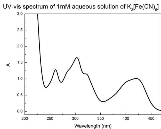
**Fig 3:** Absorption spectrum of  $K_3[Fe(CN)_6]$
