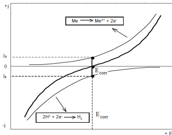
**Fig. 1:** The combination of anodic polarization curve with current density  $j_a$  (metal oxidation) and cathodic polarization curve with current density  $j_c$  (cation reduction and hydrogen depolarization). The bold line represents the sum of both processes.
