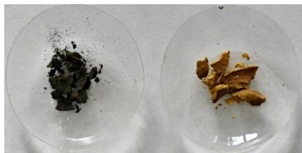
Figure 1.: Graphene oxide – two different products; Left (F3) from -20+100 mesh graphite flakes; Right (F1) from -200 mesh graphite flakes.
