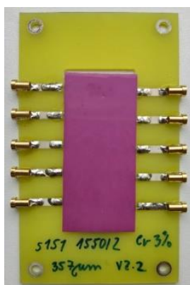
Fig. 1: Alumina ceramics doped with 3% Cr 2 O 3 equipped with electrode system and placed on holder with connector for HV.
