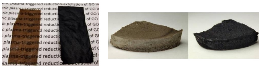
Fig. 1: GO paper before and after the fast (<1s) plasma reduction; 3D aerogel-like GO and rGO samples (GO is left and rGO right).
