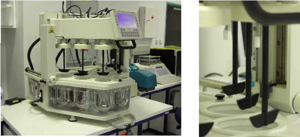
Figure 9.12. A sectional view and a photo of a USP 2 dissolution apparatus (dimensions in millimeters).
