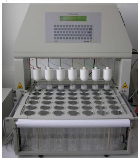
Figure 9.14. A sectional view and a photo of a USP 3 dissolution apparatus (dimensions in millimeters).
