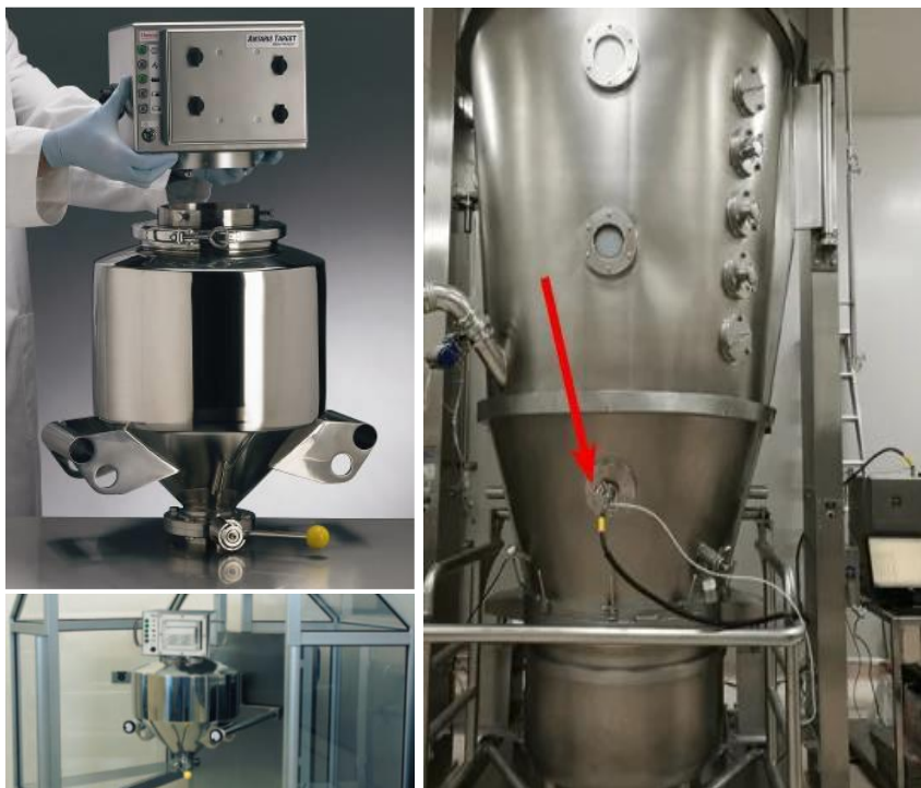
Figure 2.25. NIR analyzers connected to a homogenization apparatus. Integration of in-line NIR analysis in a fluid bed dryer.
