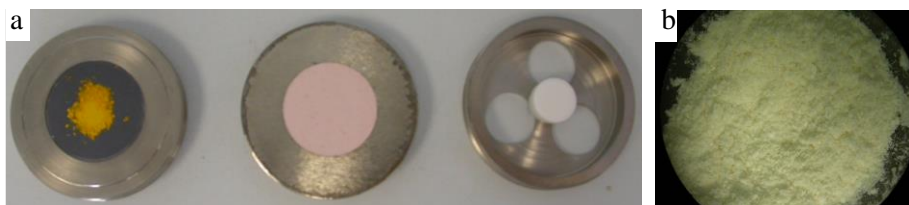
Figure 4.24. Samples prepared for measurement, placed in the most used holders in the X-ray powder diffraction with Bragg-Brentano geometry (a), raw powdered sample (b).
