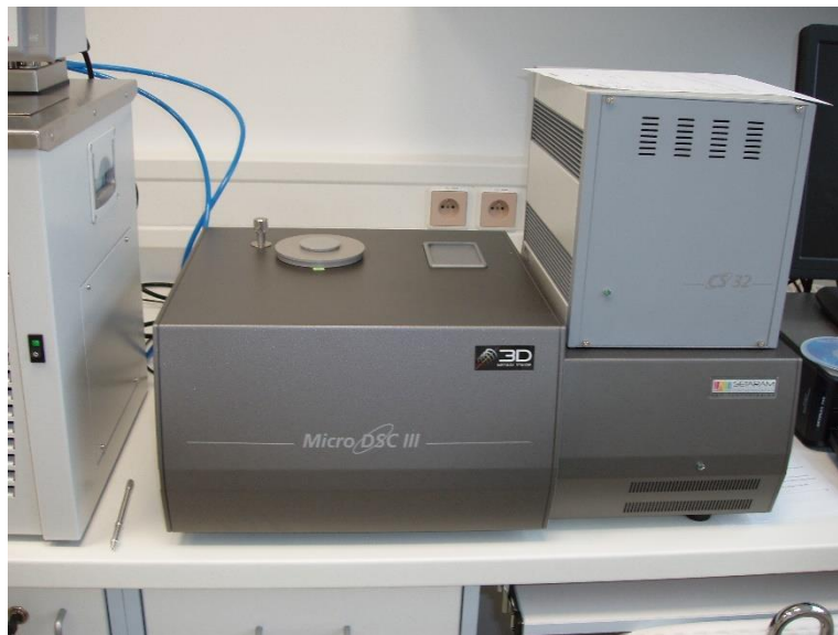
Figure 8.13. Micro DSC by SETARAM (from left: external cooling, unit with a calorimetry block, and CS 32 unit for collection and data transfer to PC).
