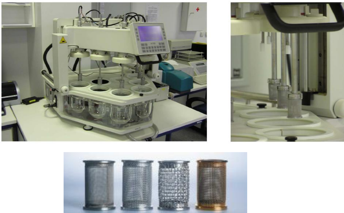
Figure 9.11. A sectional view and a photo of a USP 1 dissolution apparatus (dimensions in millimeters).
