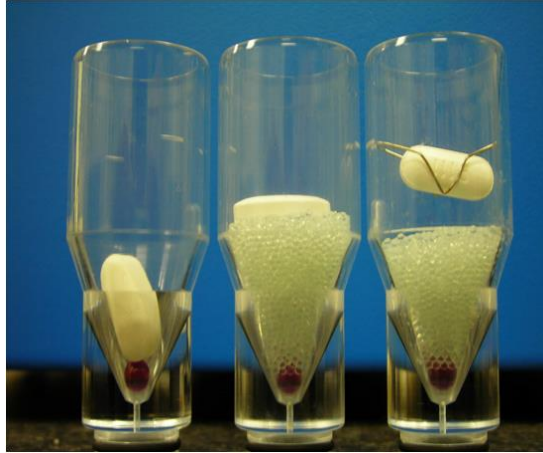
Figure 9.15. A sectional view and a photo of a USP 4 dissolution apparatus: large cell for tablets and capsules (upper picture part), tablet holder (dimensions in millimetres).
