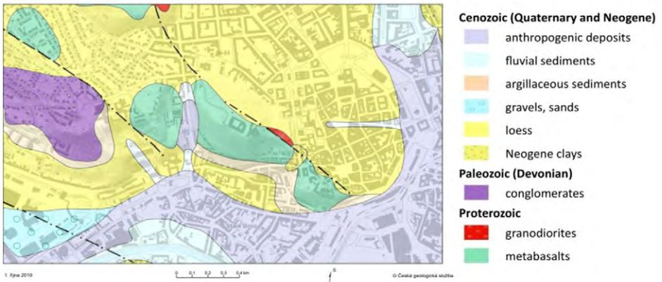
*Fig. 2: A geological scheme of the city centre with Špilberk and Petrov Hills which correspond with occurrences of metabasalt outcrops.*
