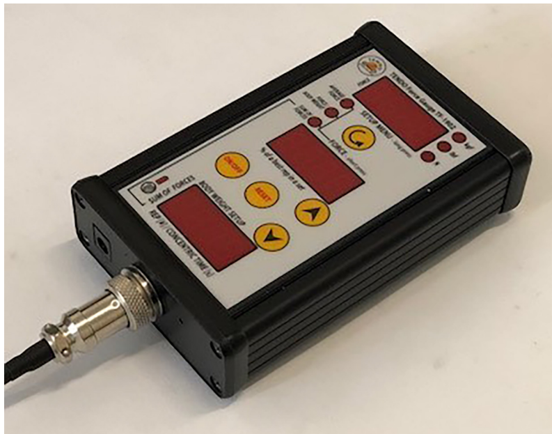
Figure 2 Tendo Force Gauge
