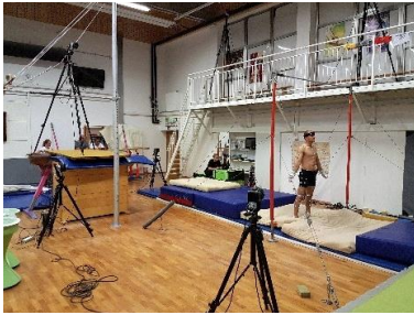
Figure 3. Positions of 7 QTM cameras
